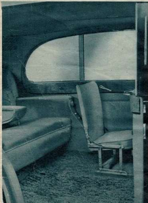
With two fold-down occasional seats and the three-passenger front seat the total seating capacity is eight. Not only is there ample leg room for the occasional seats, but also their use does not in any way incommode the main seat passengers. Both the driving side window and the partition are electrically operated. The rear window blind is also controlled by a touch of a switch.
