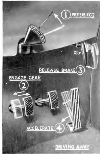
Fig. 4 Operation of Controls for Driving Away
