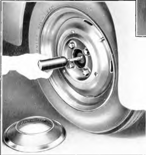
Fig. 34 Lubrication of Hubs
