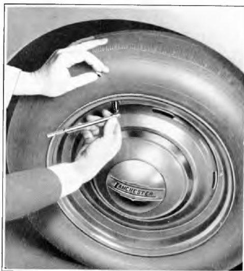
Fig. 35 Taking Tyre Pressure
