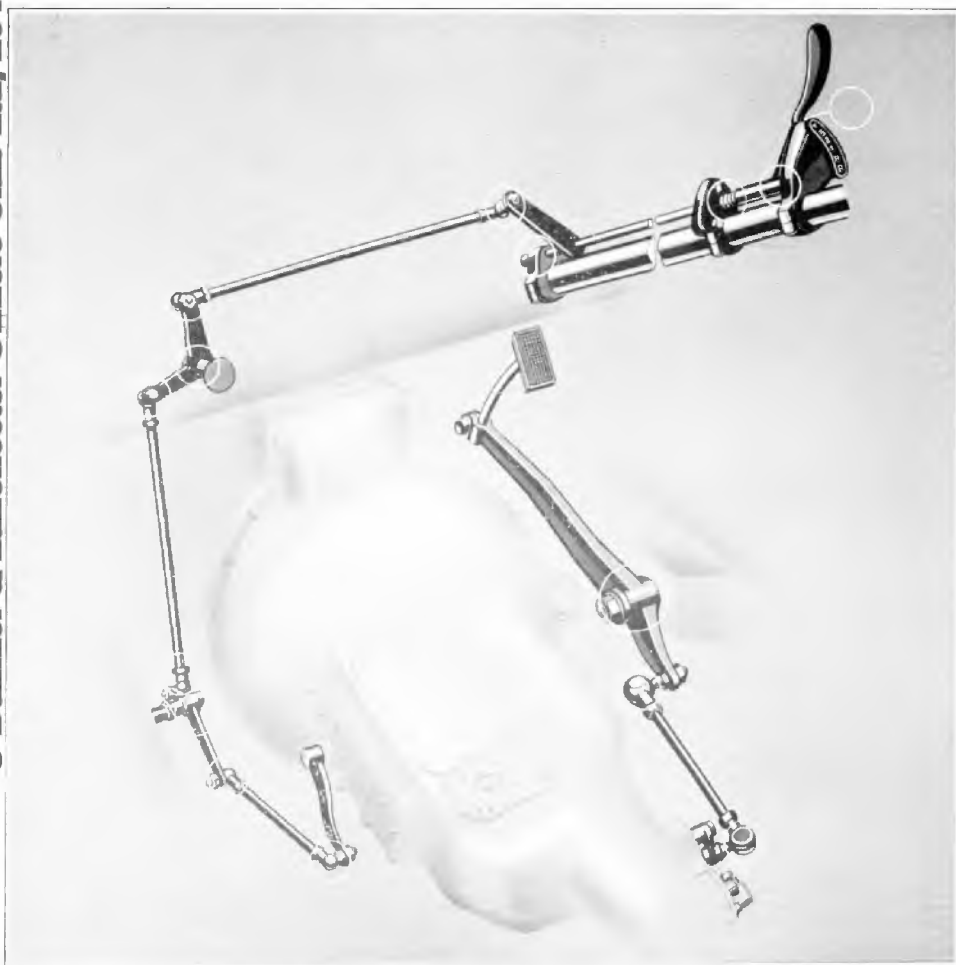
Fig. 28 Gearbox Selector and Operating Controls. Lubricate.
