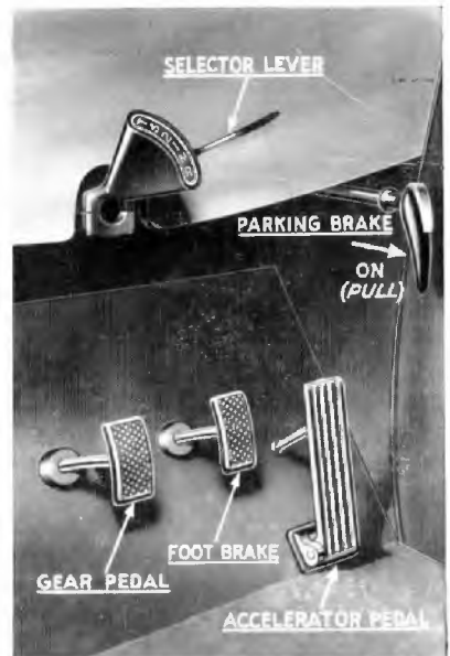
Fig. 3 Identification of the Driving Controls
