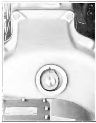
Fig. 11 Valve Timing Mark
