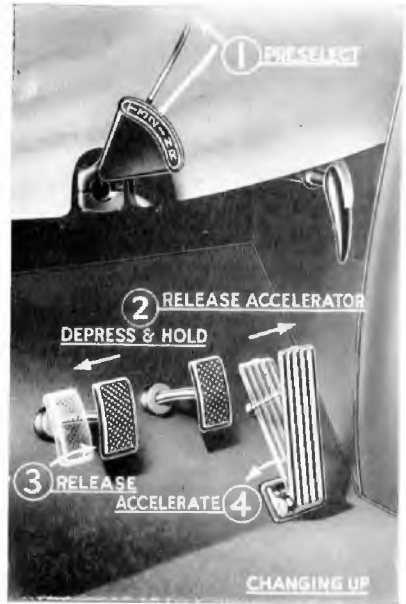
Fig. 5 Operation of Controls for Changing Up
