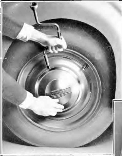
Fig. 34 Lubrication of Hubs
