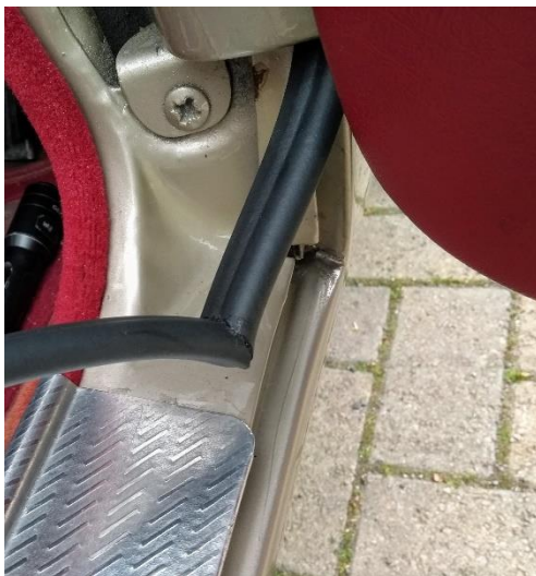
Fig 9 – the join at Point D before the lower A Post seal is stuck down.
