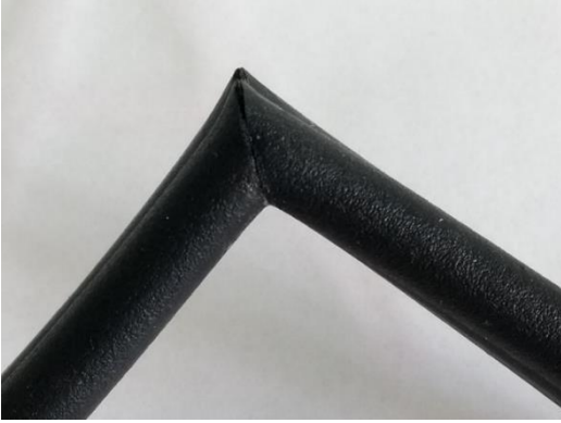
Fig 5 – The first 2 lengths of seal mitred and joined at 90° with super glue.
