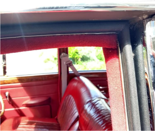
Fig 6 – the seal once in place at Point A (note that it is reflected in the chrome B Post finisher; there aren't 2 seals!).
