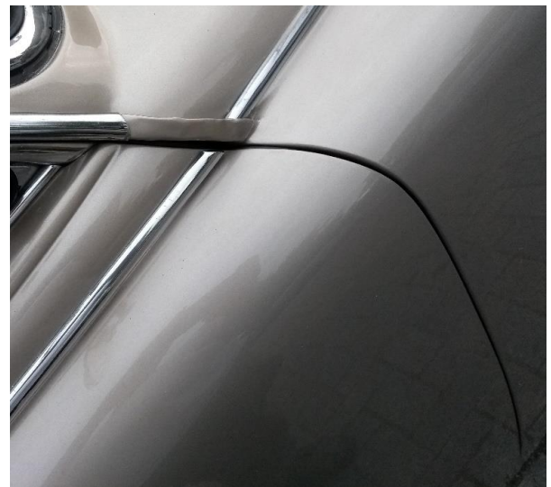
Fig 12 - The A Post seal with the door closed.
